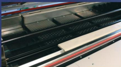
Cooling zone with integrated bottom cooling of the VisionXP+
